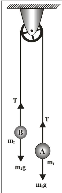
are connected by a string which passes over a frictionless pulley if  $m_1 > m_2$  then body **A** move downwards and body **B** move upwards with same acceleration as shown in fig
